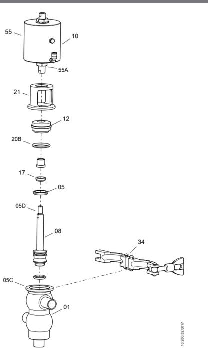
12. Open and close the valve several times applying compressed air to the actuator to make sure it operates correctly and the shaft seal fits smoothly with the valve body.
